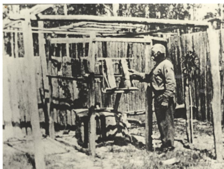
Giacomo Piccoli demonstrating his bush built hand reeling machine. Photo courtesy New Italy Museum
